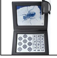
**Purpose:** To assess binocular function at a close distance.
